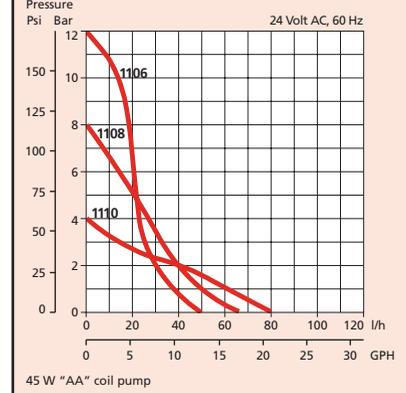
Note: Characteristics with water at 20 °C - Figures of flow are averages.
